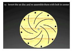
Separate the two discs and remove the panel pins. Reverse the front disc and place it against the back disc so that the routed arcs cross each other. Fit the axle bolt and adjust so the discs move easily
